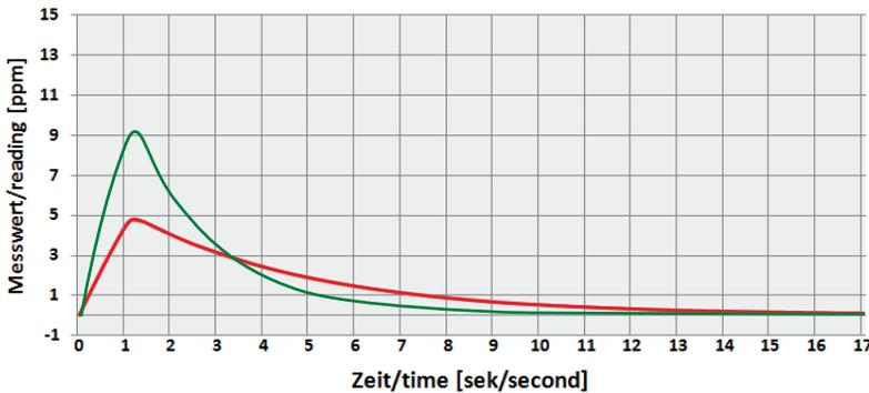
\* A comparison of the reaction time is carried out with the so-called  $T_{90}$  value. This value shows how many seconds it takes to reach 90% of the measured value.
